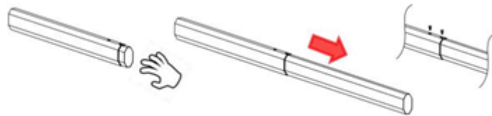
Figure 1 Connect the main boom with the Secondary arm together by 2 screws
